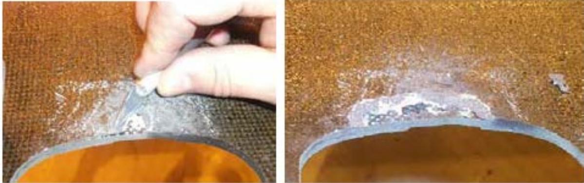
During the composite lay-up production process, the requirement is to remove the protective plastic cover from the composite plies, which should be removed in one piece. Due to the thin nature of this protective material, it can easily tear and there is a risk that pieces could remain on the composite surface, causing FOD by inclusion.
