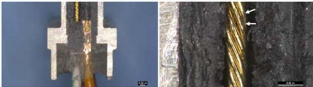
Figure 1 (left) – Partially decapsulated pin inside Micro-D connector
